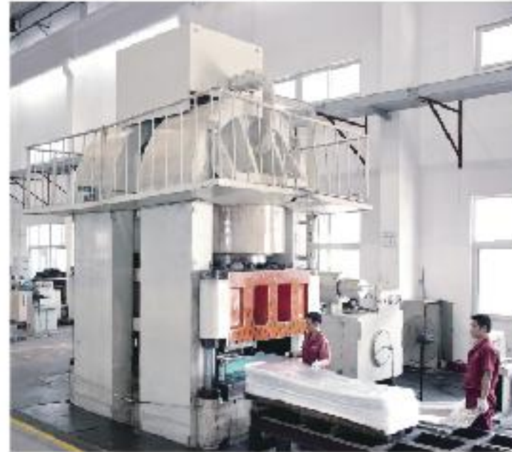
Pressure Press load of 20,000 tons
